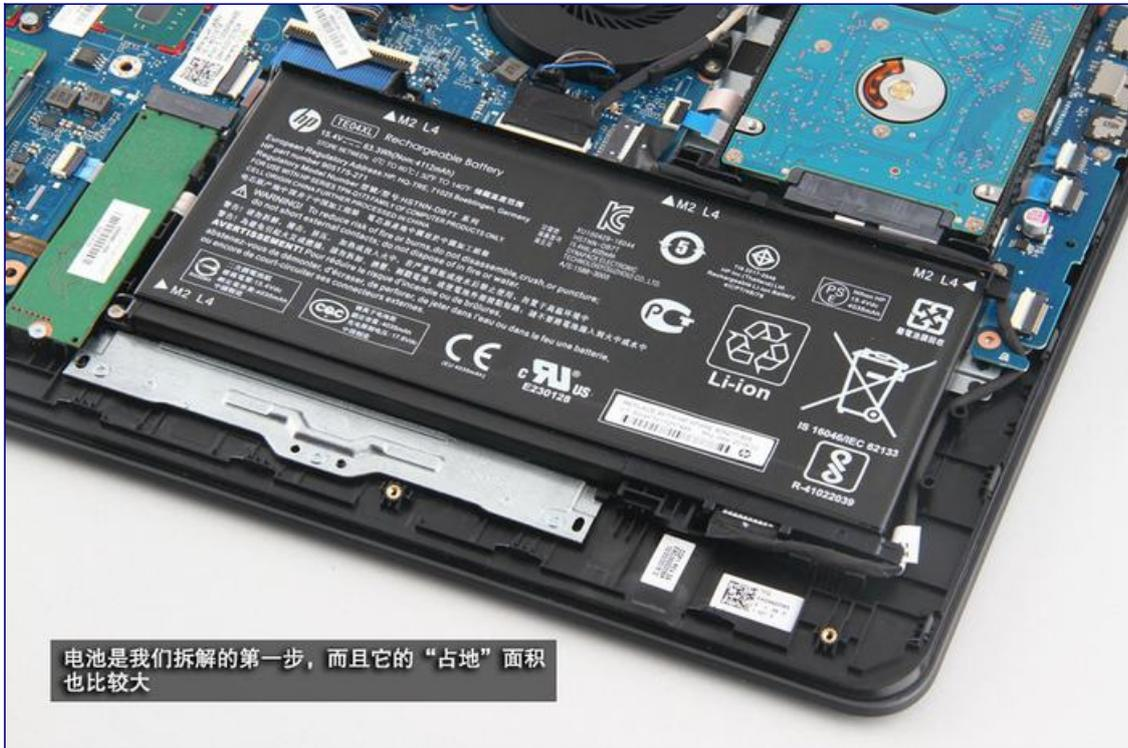
The HP Omen 15 comes with a 15.4V, 63.3Wh, 4112mAh Li-ion battery, HP P/N: HSTNN-DB7T.
