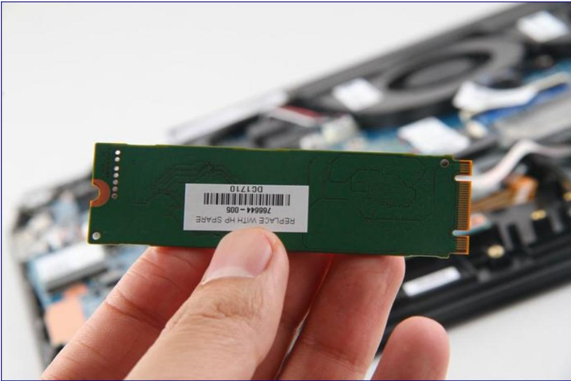
Samsung MZ-NTY1280 CM871a 128GB [M.2 SSD](#), speed evaluation: Read 535M/S, Write:515M/S (This is the Samsung official specifications, the actual speed may have some difference due to the use of the scene and Device configuration).
