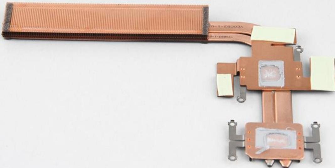
The heat sink and the copper tube are connected together. This advantage is more conducive to heat dissipation.
