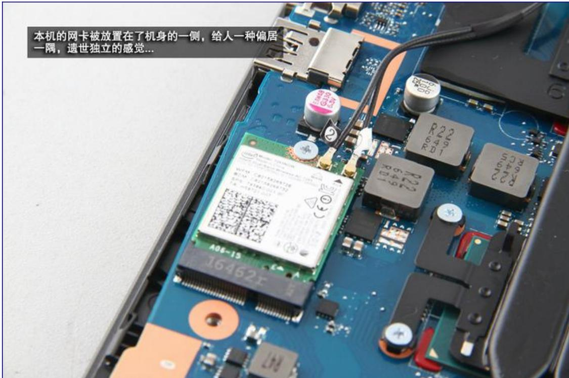
Intel Dual Band Wireless-AC 7265NGW wireless card, it supports 802.11ac, 2 x 2 Wi-Fi\* and Bluetooth 4.0.
