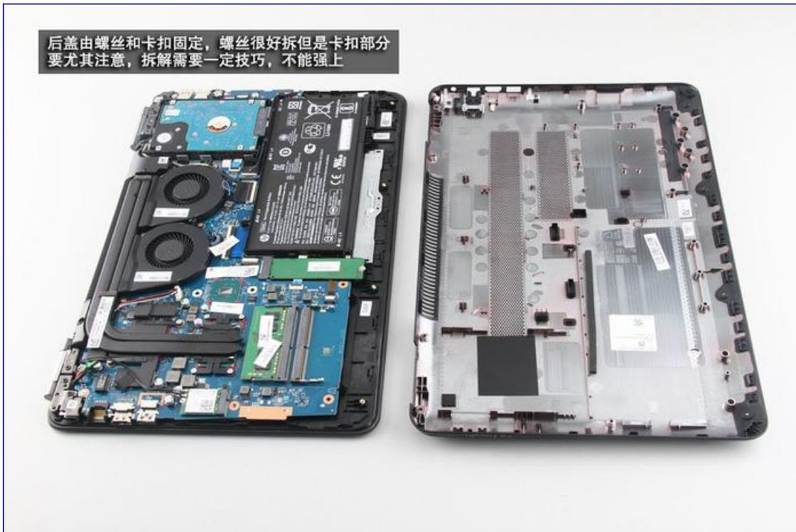
With the back cover removed, you can get access to the battery, SSD, RAM, Wi-Fi card, hard drive, cooling fan and heat sink.
